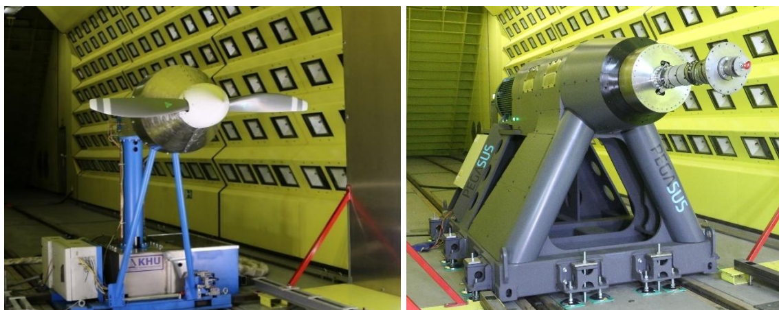
Figure 26: Standard configuration of the Prop Rig shown in the left image. Agiros test bench shown in the right image.
