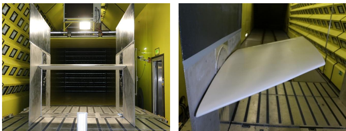
Figure 20: Test setup for a wing section test inside the IWT.
