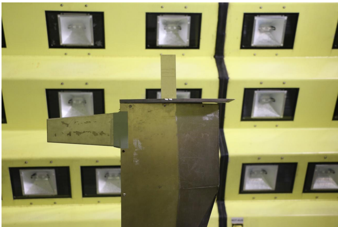
Figure 40: Icing blade installed in the test section.
