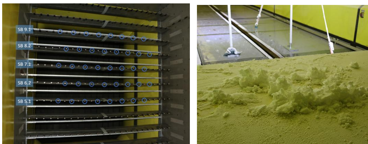
Figure 29: Nozzle setup for blowing snow tests in the RTA IWT and snow piled up.
